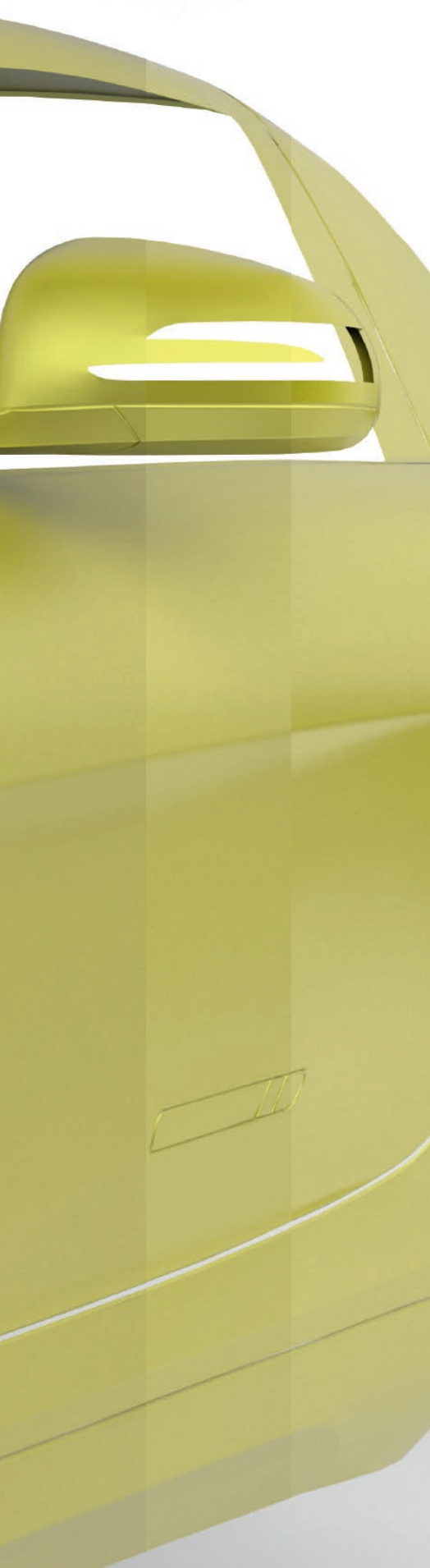
Light reflection on a glossy clearcoat (simplified illustration, as effect pigments also have a scattering effect, although only in the basecoat paint).
